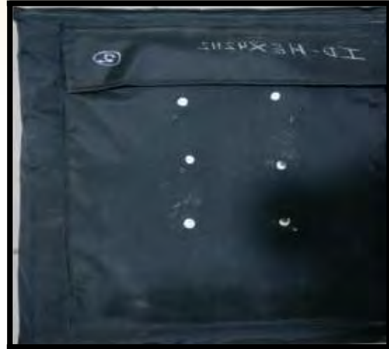
HAP+SAP tested with 7.62×39mm (HSC)
