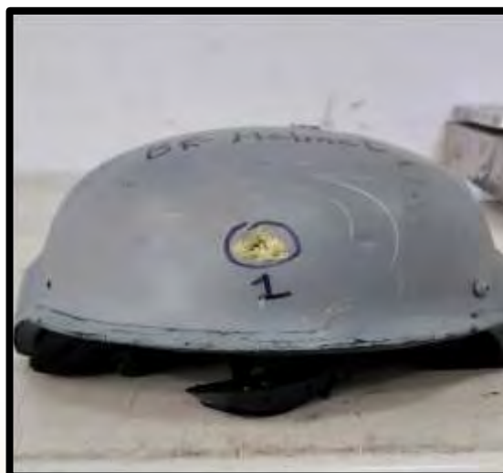
Bullet Resistant Helmet tested with 9×19mm
