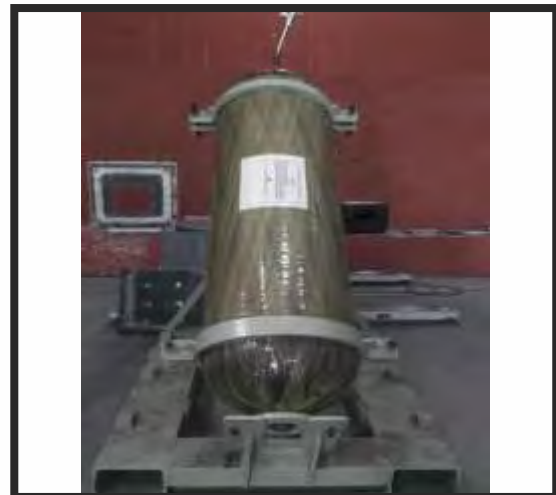
Cylinder tested with 7.62×51 mm API
