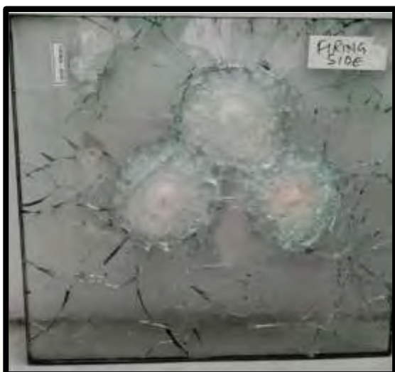
Bullet resistant Glass tested with 7.62×51mm
