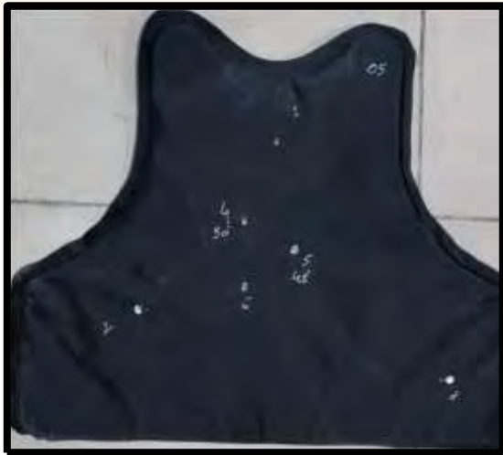
Soft Armor Panel tested with 9×19mm
