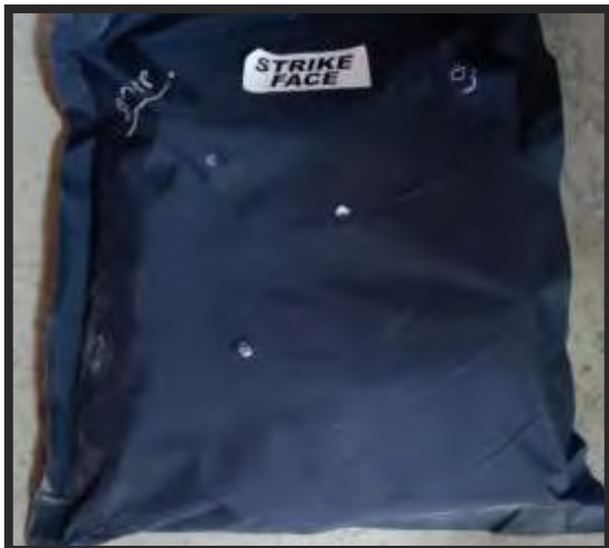
Groin SAP tested with 9×19mm
