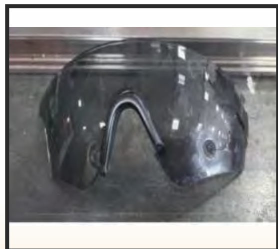
BR Goggles tested with 12 bore
